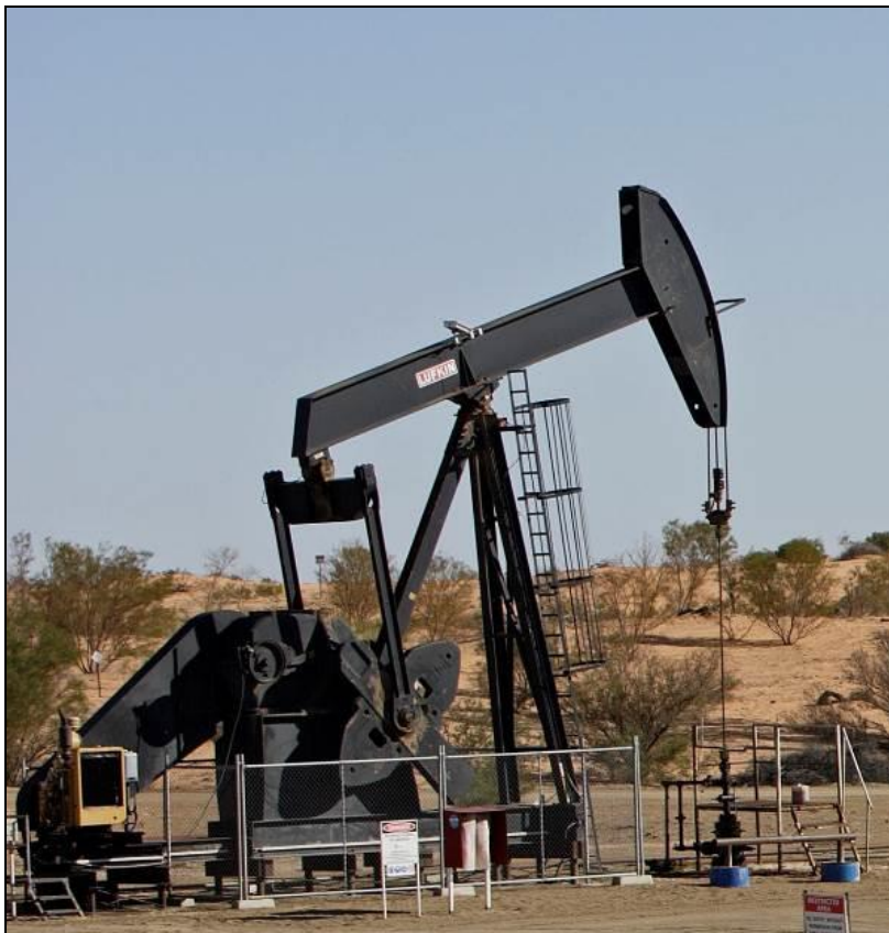
Plate 1: Rod pump operated by beam pump unit
